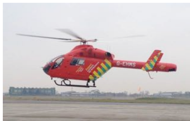
No tail rotor is an important safety feature of the MD902
